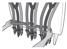
3 Once the Connector Strap is properly positioned on the school bus seat back cushion, tighten the cam wrap straps for the middle STAR restraint first and then the two outside STAR restraints.
