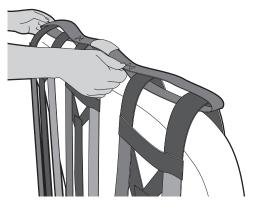
Check to be sure the Connector Strap is centered on the seat back cushion. This will prevent the outside straps from sliding off the ends of the seat.
