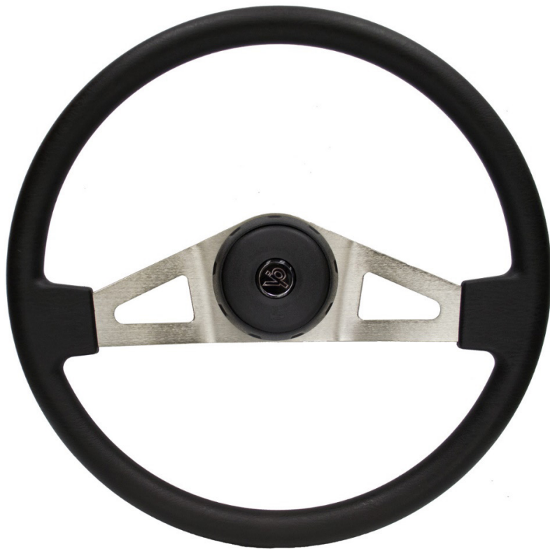
Shown above: polyurethane molded foam grip with brushed nickel plate spokes
