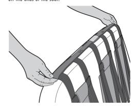
Position three STAR restraints on the 39" school bus seat before connecting the cam wrap straps. Thread the cam wrap straps through the three Connector Strap loops.
