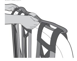
Check to be sure the Connector Strap is centered on the seat back cushion. This will prevent the outside straps from sliding off the ends of the seat.
