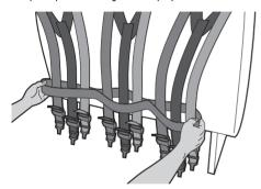
Once the Connector Strap is properly positioned on the school bus seat back cushion, tighten the cam wrap straps for the middle STAR restraint first and then the two outside STAR restraints.
