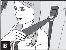
3. Place the lap-shoulder belt over the shoulder and around the passenger's upper body. **C**
