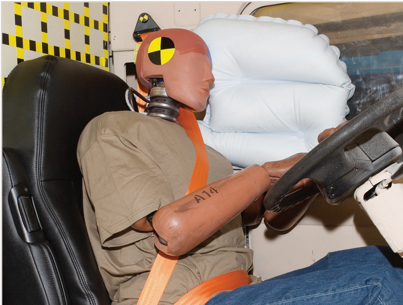
IMMI tests RollTek on a 90° rollover machine at CAPE®.
