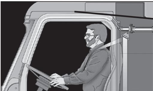
Cut above or below stowed airbags & inflator cylinder
