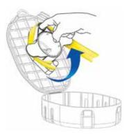
Place loop end over knob and rotate to wind web.
